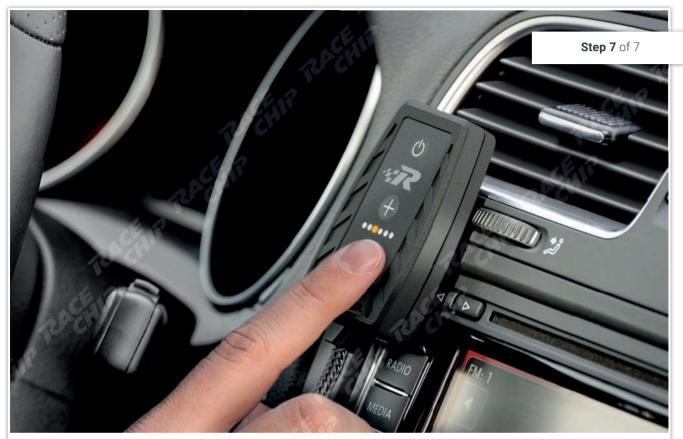
Start your engine and shift to neutral. Please also check that the RaceChip Response Control unit is operational by pressing the On/Off button. If the first orange LED on the keypad lights up, then the RaceChip Response Control unit is operational. Next, depress the accelerator pedal to check the throttle response. The installation process is now complete. We wish you happy driving!
